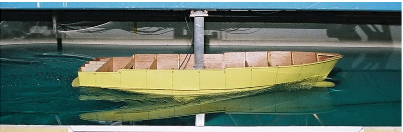
Model testing at 12 knots
